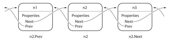
To add a node to the list, disconnect the existing nodes in the list, insert the new node, and reconnect the nodes appropriately. Here are the basic steps:
